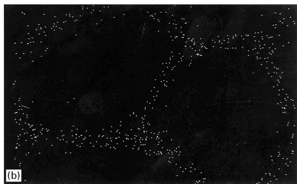
Figure 4 Typical SEM micrographs of a sample doped with 0.78 mol% BaO, sintered at 1300 °C. (a) SEM micrograph; (b) EDS elemental scan for Ba.
